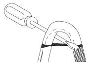
**6** While bending the heater cable, work it through the braid opening.
