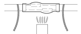
Center the 152mm (6") length shrink tube over the connectors leaving the braid straps exposed. Shrink with heat gun until completely shrunk. A uniform bead of glue should appear around the ends of the shrink tube.
