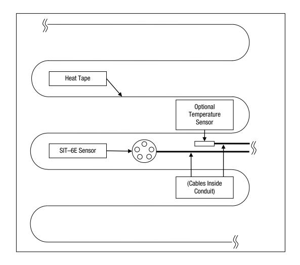
Figure 3. REPRESENTATIVE SIT-6E PAVEMENT INSTALLATION
