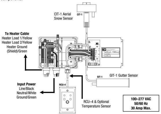
Figure 2. REPRESENTATIVE GF Pro SYSTEM SCHEMATIC
