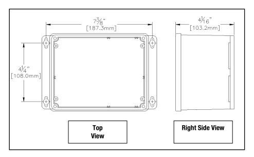
Figure 1. GF Pro MOUNTING HOLE FOOTPRINT
