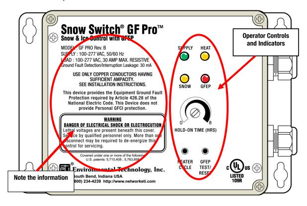
Figure 5. THE GF Pro FRONT PANEL
