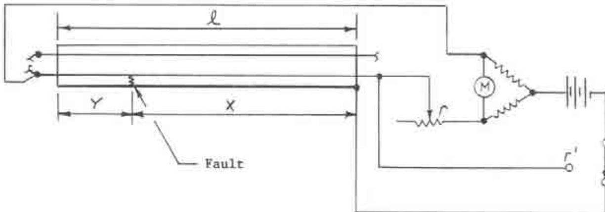
The following is a detailed instruction set on how to use the Biddle fault locator on M.I. cable.
