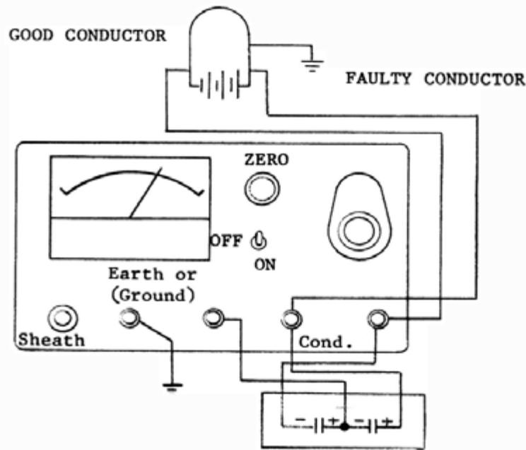
FIGURE 5: A method of overcoming electrostatic charges
